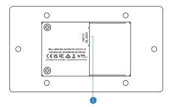
• HDBaseT™ Input - RJ45 HDBaseT™ port to connect to the HDBaseT™ input port of the compatible Blustream HDBaseT™ transmitter / matrix device
