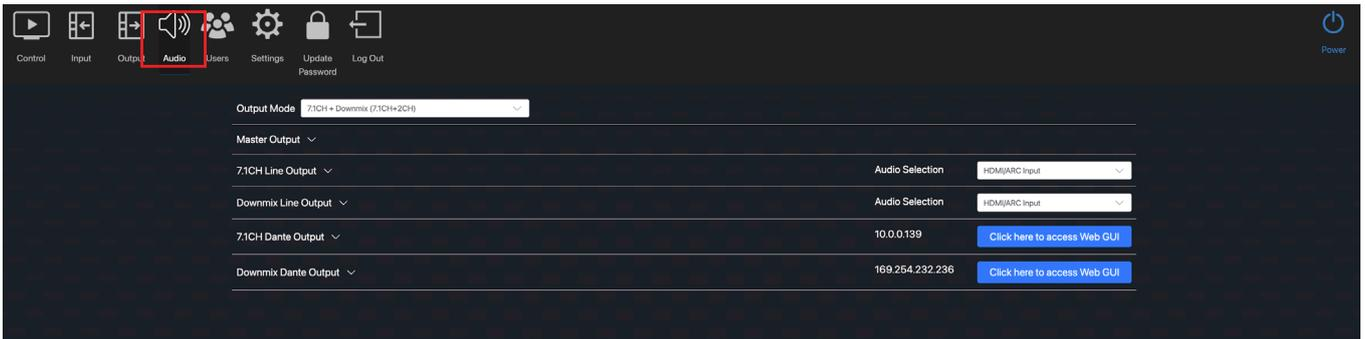
The first main setting is to decide how the SW42DA will decode audio subject to the installations requirements. The Output Mode displays the current format selected. To change the audio output mode, simply select the desired format from within the drop-down box. These are:
